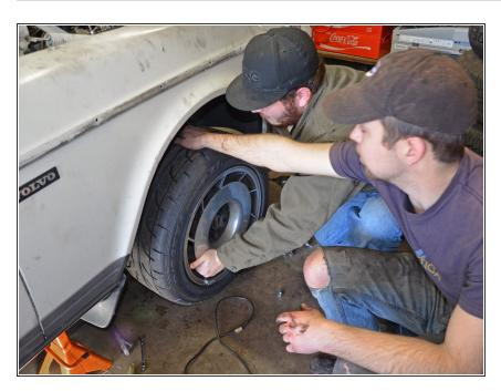
Install your new wheels over the lugs of the wheel adapters and tighten the lug nuts to 85 ft-lbs.
