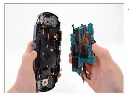
• Completely separate the motherboard from the case. Set the case aside.
