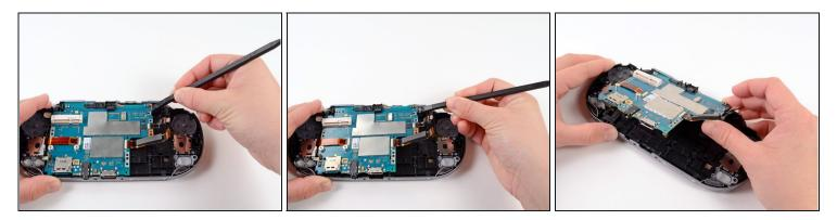
• Starting at the upper right hand corner, use a spudger to gently lift the motherboard out of the casing assembly.
