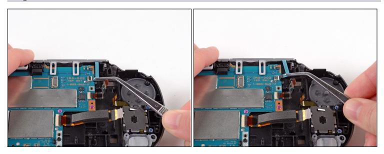
• Using <u>tweezers</u>, gently pull the blue power flex cable out of the socket, and rest it out of the way.
