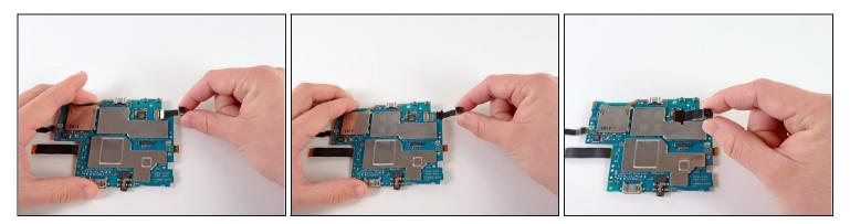
• Gently pull the rear camera out of the flex cable socket.
