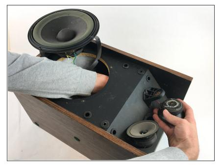
• While holding the tweeter, use your other hand to feed the wire through the hole at the bottom of the tweeter mount.
