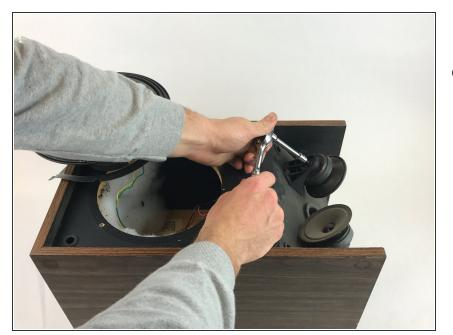
Using the socket wrench and the 1/4" socket, unscrew the 12.5 mm bolt that mounts the tweeter to the bracket.
