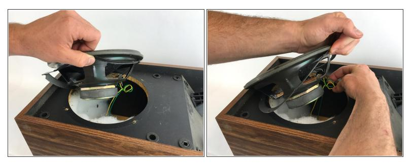
• Untwist the slack in the wires that are connected to the main speaker.
