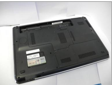
Carefully pull out the battery while holding the latch to the open position with your finger.
