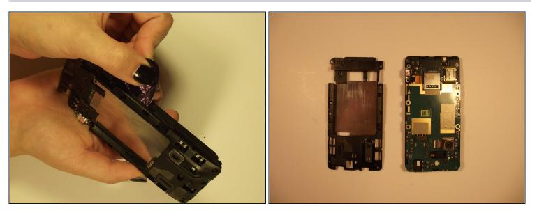
• Remove the rear housing by prying around the edge with your Safety Pry Tool
