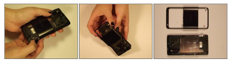
• To remove the remaining cover, lift the side port, which was previously uncovered, then lift the outer shell from the bottom of the phone and slide it forward
