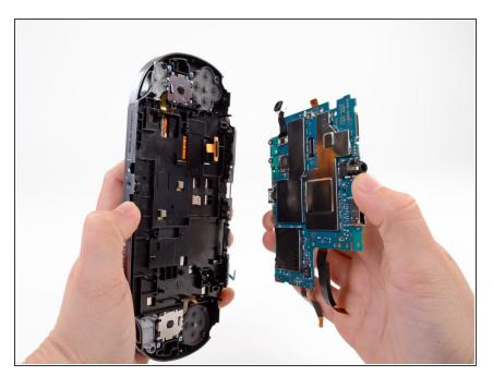
Completely separate the motherboard from the case. Remove the case.
