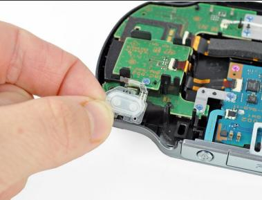
Using a spudger, gently peel up the left shoulder button from the light adhesive connecting it to casing.
