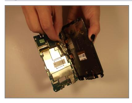
• Disconnect the two aluminum flex cables
