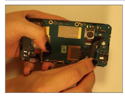
• Unplug the wire connecting the vibrator to the board with your tweezers
