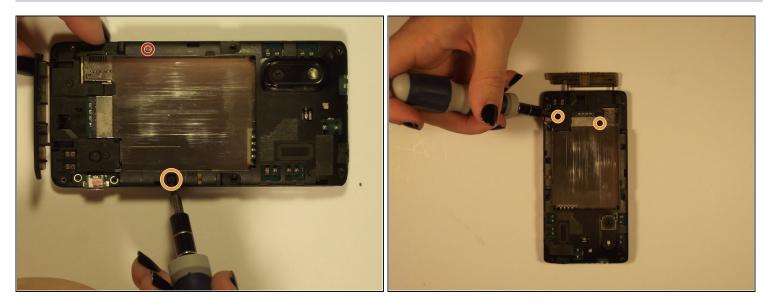
• Remove the two revealed screws on the outside (Torx = red, Phillips = orange), and then remove the two phillips on the bottom of the phone
