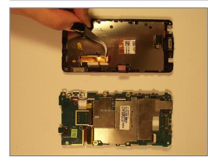
• The flex cables should be the only binding and after being removed should leave you with the separate screen
