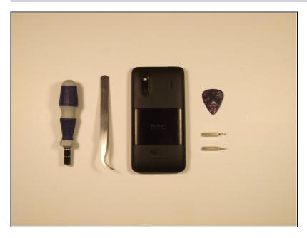
Tools: Phillips #000 Screwdriver, T4 Torx Screwdriver, Safety Pry Tool (Guitar pick), Tweezers
