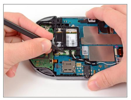
Using the pointy end of the spudger, gently pry the GPS antenna cable off the wireless card.
