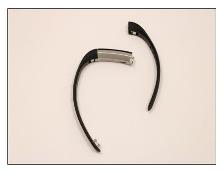
Slide the band up to release it from the Fitbit Alta tracker. Then, repeat on the other side to remove the band.
