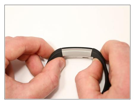
To release a latch, press down on the flat metal button holding the band to the Fitbit Alta. Pull up on the latch to release the band from the body.
