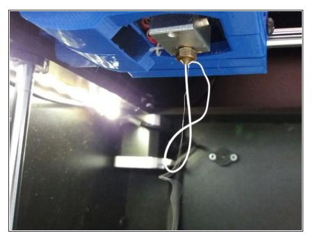
Push the filament through the PTFE tube until it exits through the nozzle to make sure it has been inserted all the way.
