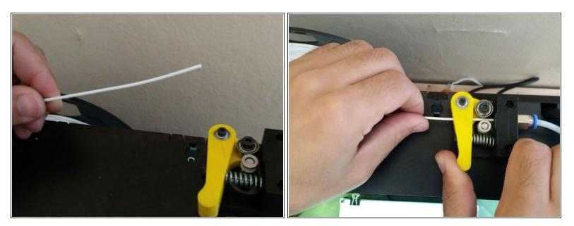
Press the ear of the extruder with one hand and insert the filament into the hole as shown in the pictures.
