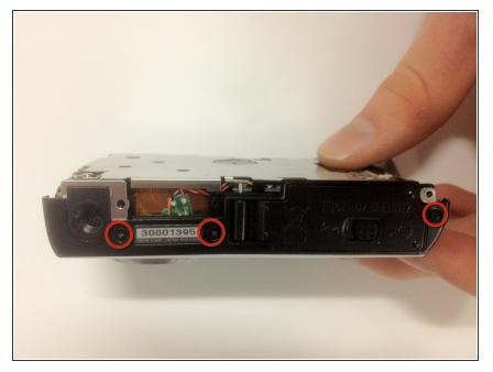
Remove the three 3x3mm screws that attach the front casing to the bottom.
