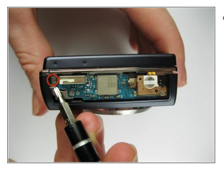
Remove the 3x2mm screw underneath the panel near the top of the camera.
