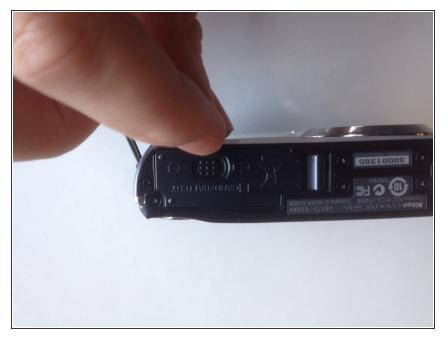
• On the bottom right of the camera, locate the battery flap switch.
