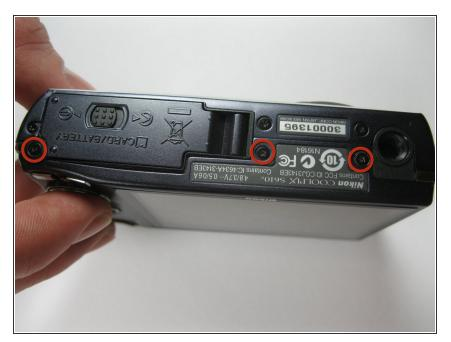
• Remove the three 3x3mm screws attached to the rear casing.
