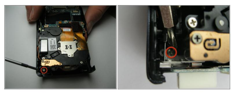
• Remove the final 4x3mm screw at the top of the camera near the lens.
