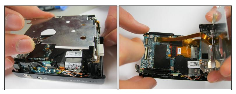
• Lift the back panel off the motherboard.
