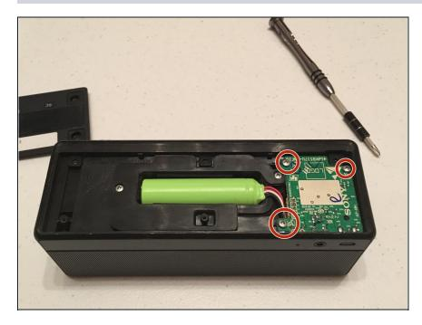
Remove the 3 philips head screws holding in the green circuit board
