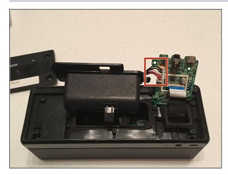
• Unclip the battery pack and replace it with another one.
