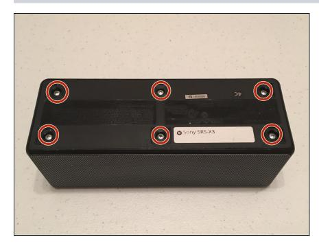
• Remove the 6 philips head screws using the PH1 bit.
