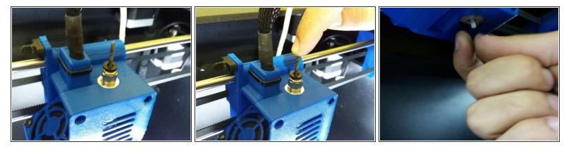
By positioning the drill bit into the indicated hole, push it down until the inner PTFE comes out from under the head (where the nozzle hole is).
