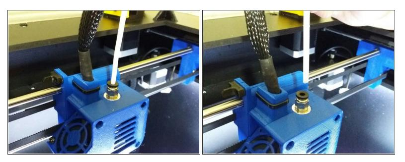
With your hands, pull out the PTFE tube from the printhead by pressing the black piece of the part where the tube is seated
