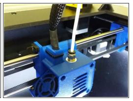
Replace the nozzle at the bottom of the printhead and the PTFE at the top, pushing it all the way with your hands.
