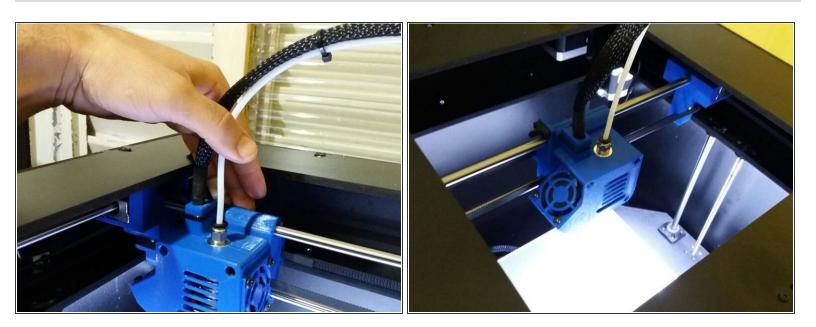
With the table in position push the head manually toward the machine center in order to obtain an easy handling.
