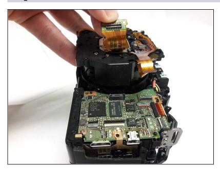
• Pull the lens, the entire piece to the left of the motherboard, out of the camera.
