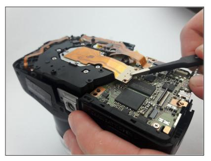
• Use <u>tweezers</u> to pull the large ribbon cable connecting the back of the lens to the motherboard.
