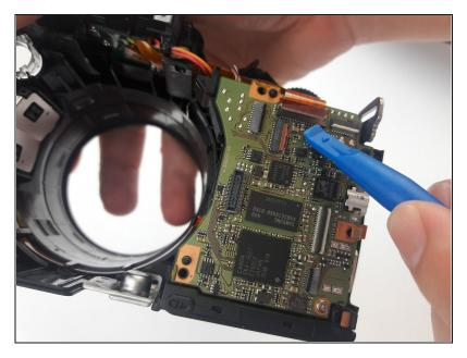
• Remove the ribbon cable on the top of the motherboard with a plastic opening tool.
