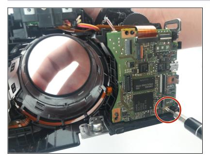
• Using a PH000, unscrew the 3.5 mm screw on the bottom right side of the motherboard.
