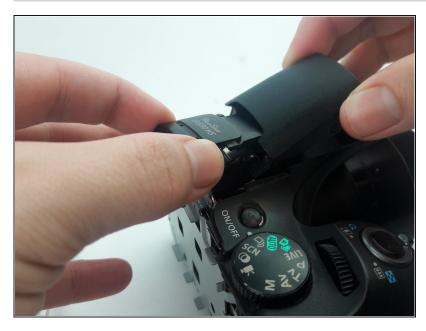
• Lift the shutter light and pull the shutter back panel off the camera.
