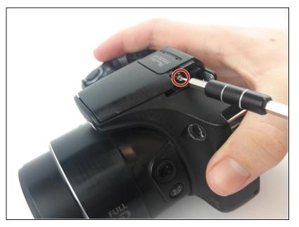
Remove the two screws (5-6mm) on the left and right side of the shutter panel with a Phillips PH000 screwdriver.
