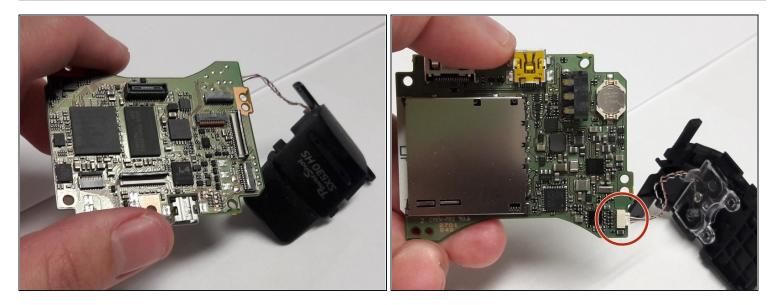
• Remove the white box on the back of the motherboard that connects the shutter's wires to the mother board.
