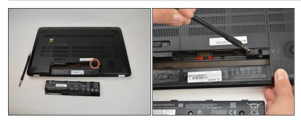
• Use a PH1-screwdriver to loosen the 7mm screw. The screw will not fully come out as it is held by a washer underneath but will come out enough to open it.
