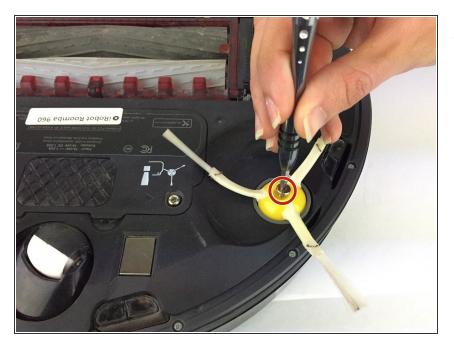
With the Flathead 2.5mm screwdriver remove the 7.9mm screw from the side-brush.
