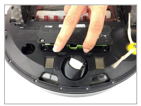
• Lift the plastic cover to access the battery.
