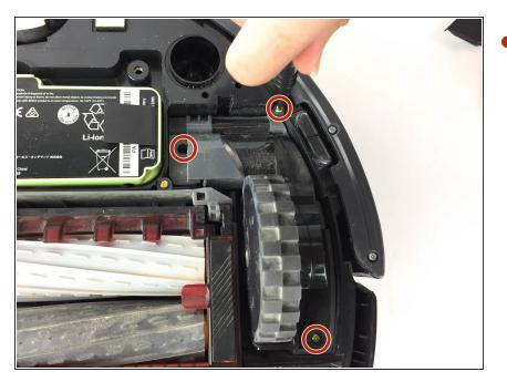
Using a Phillips #1 screwdriver, remove the three gold 15.5 mm screws.
