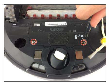
• With the Phillips #1 screwdriver, remove the two 11.4mm screws.
