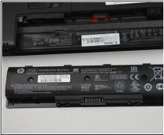
• Pull the battery out and let go of the battery slider.
