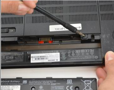
Use a PH1-screwdriver to loosen the 7mm screw. The screw will not fully come out as it is held by a washer underneath but will come out enough to open it.
