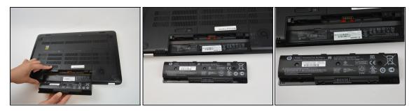
• Pull the battery out and let go of the battery slider.
