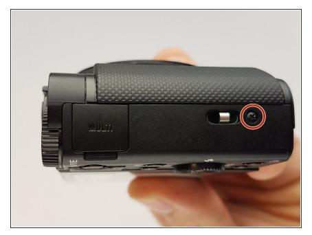
Remove the marked screw with a Phillips #000 screwdriver.
