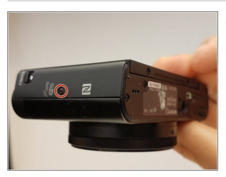
Remove the marked black M1.4 X 3.5 Phillips head screws on the side of the camera with a Phillips #000 screwdriver.
