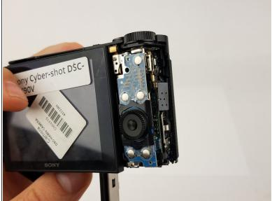
Use the plastic opening tool to remove the button board.
