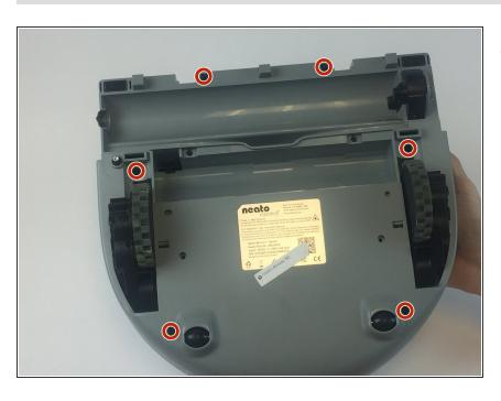
Begin by placing the robot on it's back and removing the six 11m screws using a Torx T10 screwdriver.
