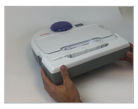
• Pull the left and right sides away from the machine to unclip the bumper. This requires that you bend the plastic a little bit. Unclip one side a little bit and allow the prong to rest on the side of the machine. Then unclip the other side and pull off the bumper parallel to both sides
