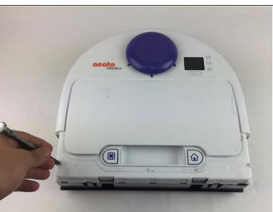
Looking from above, remove the two 11mm screws with a torx T10 screwdriver.
