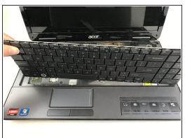
• With the top panel remove, use the spudger to lift the keyboard out of the device as shown.
