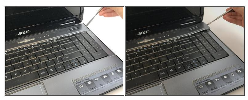
• Using a metal spudger, pry open the top panel of the device as shown.
