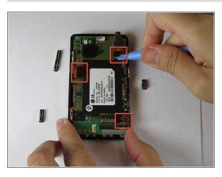
Disconnect the three ribbon connectors from the motherboard.
