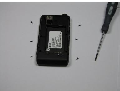
Use the #00 screwdriver to remove the six 4mm phillips screws located around the edges of the phone.
