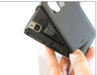
Remove the back cover by firmly pressing against the raised lip on the back panel. Slide the cover towards the top of the phone.
