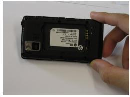
Remove the battery by placing your fingernail or a opening tool in the recessed edge and lift the battery out.
