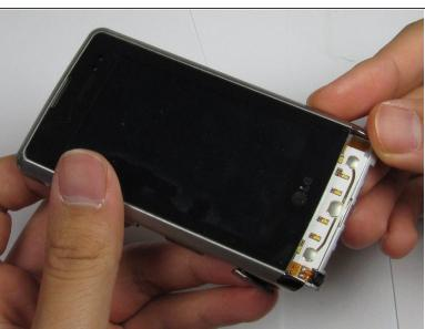
Pry the button panel from the device, starting where the screen and panel connect, until the panel detaches.
