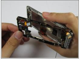
Gently separate the top of the frame from the back of the device, without completely detaching at the bottom, as shown in the third picture.
