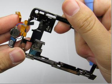
Pry the rest of the orange connector pad --on the opposite side of the device-- away from the frame, and carefully remove the entire earpiece. To re-assemble your device, follow these instructions in reverse order.
