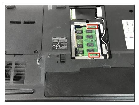
The two tabs are at the top and bottom of the case as shown.
