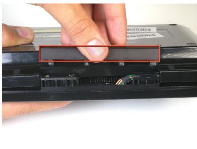
Use your hand to remove the small back cover by gently pulling upward.
