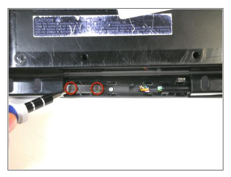
Using a screwdriver, remove the two12 mm pan head screws.
