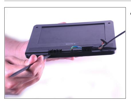
Using the spudger, separate the top and bottom covers.
