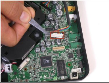
Remove the wires attached to the white base using tweezers to pull them up.
