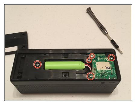
Remove 5 philips head speakers holding in the battery and the green circuit board. 2 screws holding in the battery and 3 holding the circuit board.
