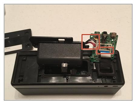
Pick out the battery pack and the green circuit board so that you can see the ribbon wire and the wire running from the battery pack to the circuit board.
