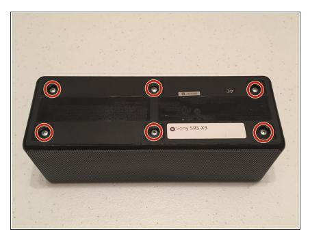
Remove the 6 philips head screws using the screwdriver and the PH1 bit
