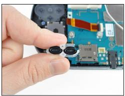
• Using tweezers, peel the start/select button off the back case.
