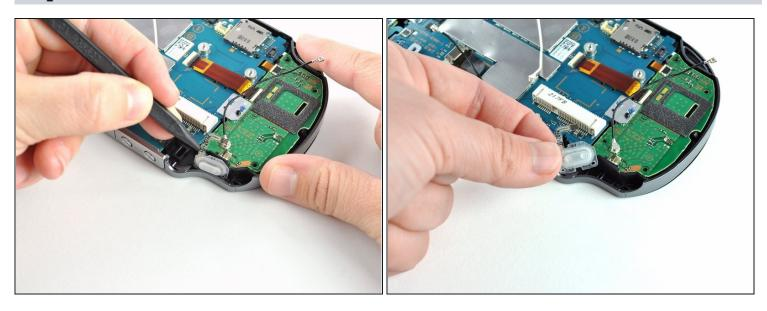
• Using a spudger, gently peel up the right shoulder button from the light adhesive connecting it to casing.
