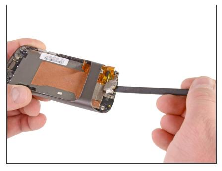
Using the spudger, pry up the trackball housing to expose the trackball assembly.
