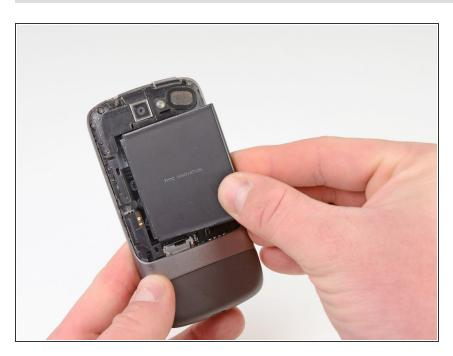
Pull the battery up and out.
