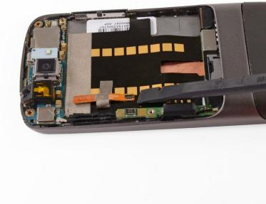
Using the spudger, pry upwards on the second microphone connector.
