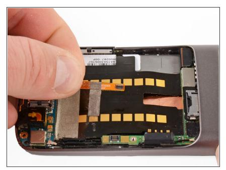
Carefully pull up on the microphone board to release the tape from the phone.
