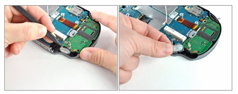
Using a spudger, gently peel up the right shoulder button from the light adhesive connecting it to casing.
