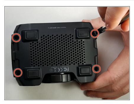
To remove the outer case, remove 4 phillips screws (Phillips #00 headtype, 9.3mm long)
