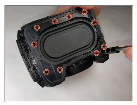
To remove the speaker cone plate, remove 10 phillips screws (Phillips #00 headtype, 9.3mm long)
