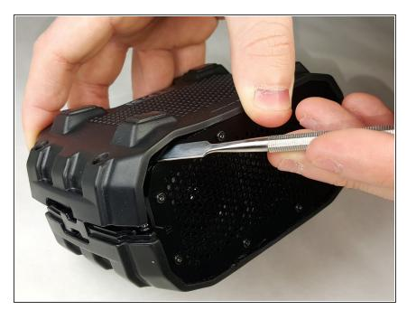
• Using a metal spudger, gently pry the side of the defective case.
