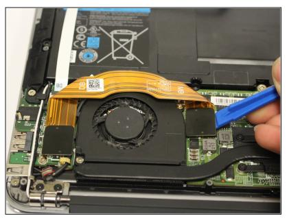
Remove the ribbons from both sides with a plastic iFixit opening tool.
