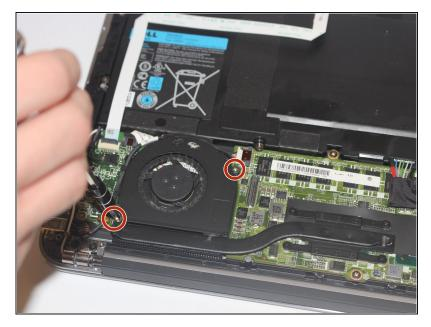
Use a PH1 screwdriver to remove the two 3mm screws that secure the fan.
