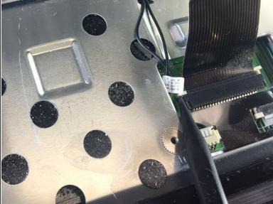
Use your plastic spudger to unlock the two white sliding connectors located on the left and right side of the device by gently pushing them out.
