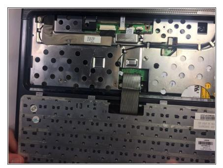
Flip the keyboard over. It may be easiest to hold it up in order to detach its wire assembly.
