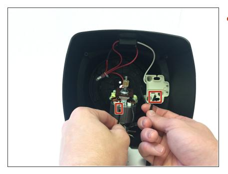
Using the wire stripper crimping tool cut the black wire connection from the power cord to the motor and then rewire the new power cord to the motor.
