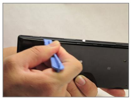
Once the part of the back cover has been opened up. Slide the spudger to pry completely detach the cover from the phone.
