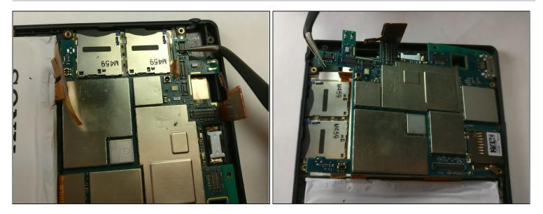
Using tweezers, carefully remove the motherboard by pulling it up and out of the backing.
