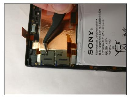
Using the <u>Tweezers</u>, carefully pry the the dual SIM slot off the sticky substance used to hold it down.
