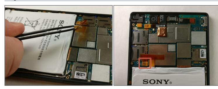
• Using tweezers, locate the battery connector and carefully pull up to disconnect it.
