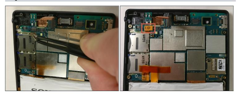
Carefully remove the SIM card connector using tweezers by gently pulling it straight up.
