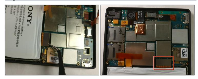
• Carefully remove the button circuit connector by using tweezers and gently pulling up.
