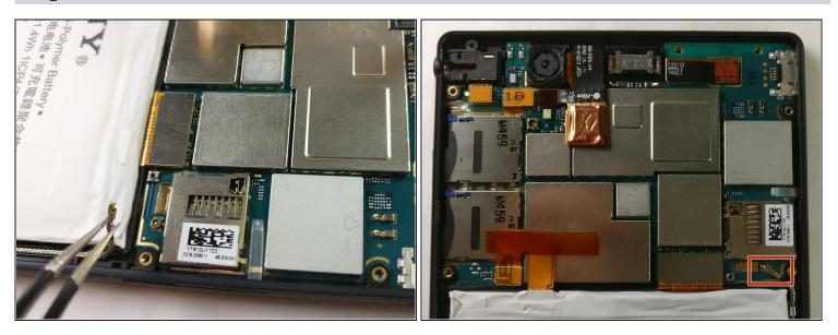
• Carefully remove the silver plug by using the tweezers to lift straight up.
