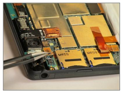
Carefully remove the audio jack by using the <u>tweezers</u> and pull firmly straight out of the motherboard.
