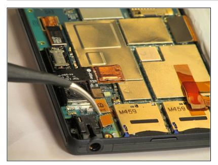
Using tweezer, locate the audio jack as shown and pull out the chip connected to the motherboard.
