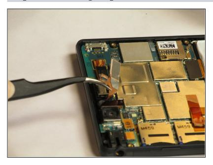
To take out the back facing camera, flip open the flap labelled 'film' to reveal the chip that connects to the motherboard.
