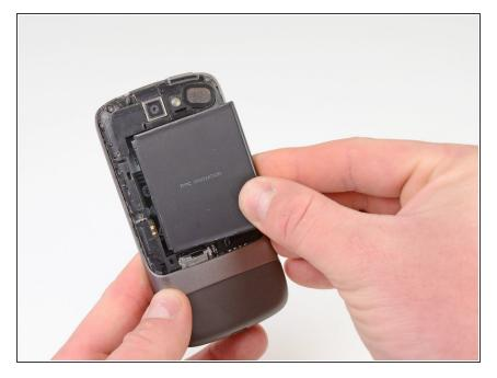
• Pull the battery up and out.
