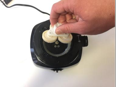
• Firmly grasp center piece of gear mechanism and pull straight upward.
