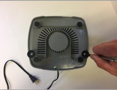
Using a #2 Phillips head screwdriver, remove the two 11 mm screws and pull the rubber suction cups straight up.
