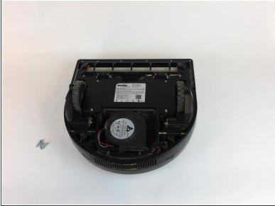
Use plastic spudger to gently pry off the external panel to expose the motor assembly.
