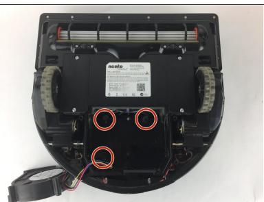
Gently lift the motor assembly straight up, out of place, being aware of the four mounting posts that hold the motor firmly in place.
