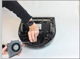
Press the tab and gently lift straight up to disconnect the motor wires.
