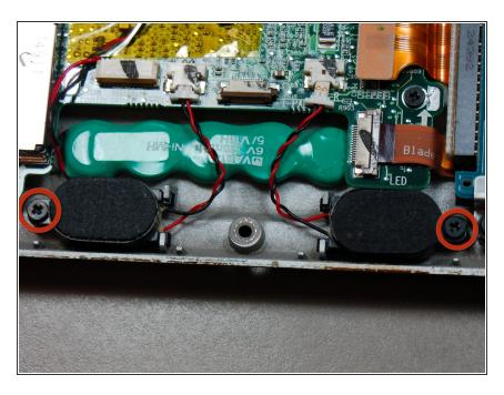
Remove the #00 4 mm screws holding the speakers in place.
