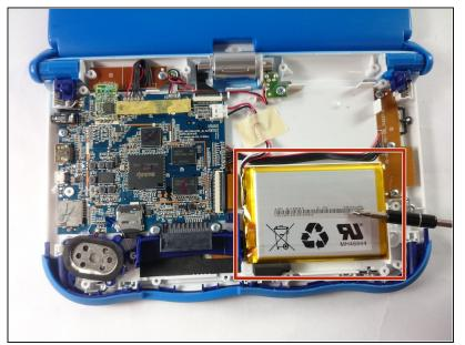
Once the back cover is removed the battery will be located in the bottom right as you can see in the image to the right.
