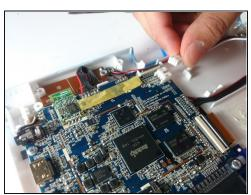
• Now that the battery is free to be moved, unplug the wire connecting the battery to the motherboard.
