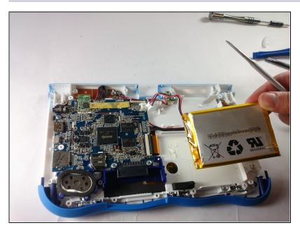
• The battery is now fully disconnected.
