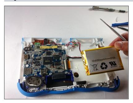
The battery is now fully disconnected.
