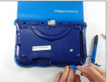
Now that all of the screws have been removed, pry the back cover off using a plastic opening tool.
