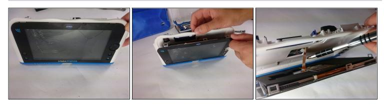
Once the pins are removed the screen should be loose from the frame and only connected by the brown film pictured.
