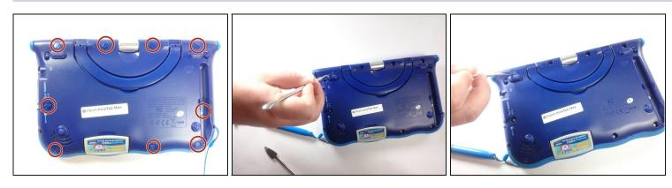
Remove all screw caps from the back panel using a metal spudger.
