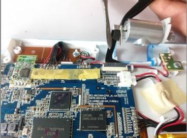
• Carefully remove the wire connecting the camera to the motherboard, using a tool to grip it if needed.
