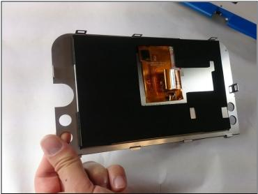
• Once unclipped from the motherboard the screen should be entirely free from the device
