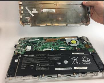
Remove the back cover by placing a prying tool in the SD slot and popping the clips out of place.
