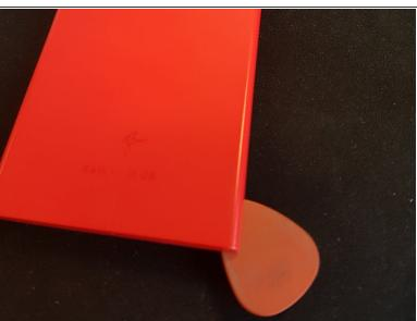
Remove the back cover, starting at the bottom right corner with your nail or a prying tool
