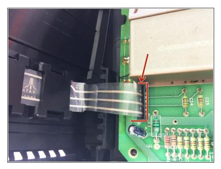
Detach the ribbon from the circuit board by gently pulling ribbon out from clip.
