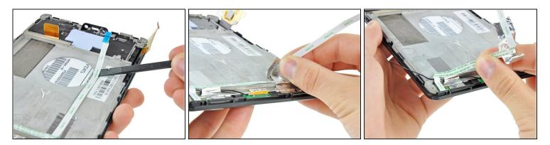
Use the flat end of a spudger to peel the ambient light sensor cable off of the frame.
