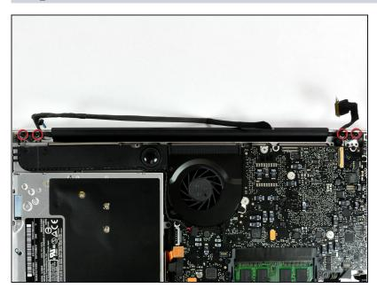
Remove the two outer 6 mm
