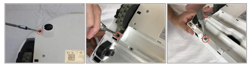
• The screws pictured here on either side of the Botvac require the extension in your tool set to be removed.
