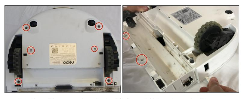
Eight 13mm T10 screws on the underside of the Botvac hold the casing together. These screws
