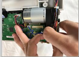
Carefully lift the top cover of the Botvac. On the right side of the Botvac is where you'll find the LCD screen connector to the motherboard. Carefully pull on the connector to disconnect it from the motherboard.
