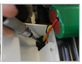
⚠ Be careful when taking out the battery. Do not pull on the wires or battery trying to get the connector out.
