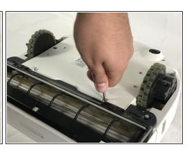
Use Phillips #1 screwdriver to unscrew the two bottom cover screws
