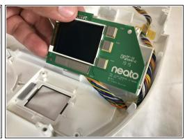
There are two 0.5cm #1 Phillips screws holding the LCD screen to the top cover. Remove these screws to lift screen off the cover.
