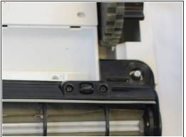
To remove the rotary brush simply grasp it firmly and pull it off.
