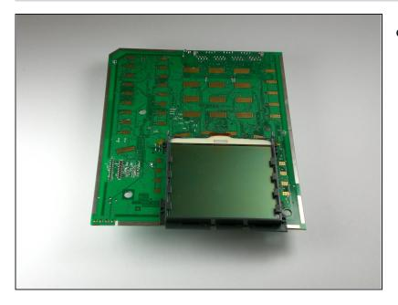
• Flip the motherboard over so that the LCD screen is facing upward.
