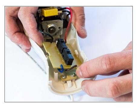
Slide out the printboard by pushing it back and forth in the clicking connection with the shell.
