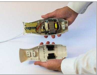
• Open up the click connections inside the shells by gently pushing the two shells together with the hand palms, right next to the gap.
