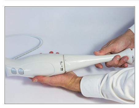
Put the lower part of blender back at the two shells by rotating it counterclockwise, as stated on the upper part.
