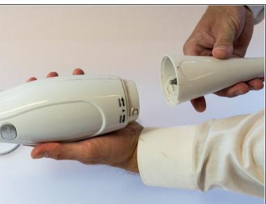
Take out the lower part of the blender, by rotating it clockwise, as stated on the upper part.
