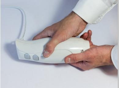
Push the two shells together until you hear a 'click' and make sure the two shells are well connected.
