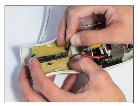
Put the printboard back into the clicking connection with the shell.
