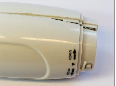
Gently put the metal spudger (1) in the gap between the two shell parts and force a small gap, so that the parts loosen up.
