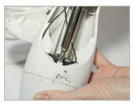
Unscrew the Phillips (2mm) connecting the middle part of the casing with the bottom part.
