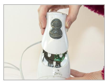
Unscrew the Tri-point screw (2mm) on the top to disassemble the top part of the casing.
