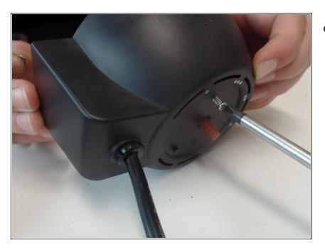
Remove the screw on the back of the body to disasemble the Voltage Capacitor from the body.
